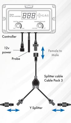
Adding the splitter cable to the controller allows you to control both inlet and extraction fans from one controller.
